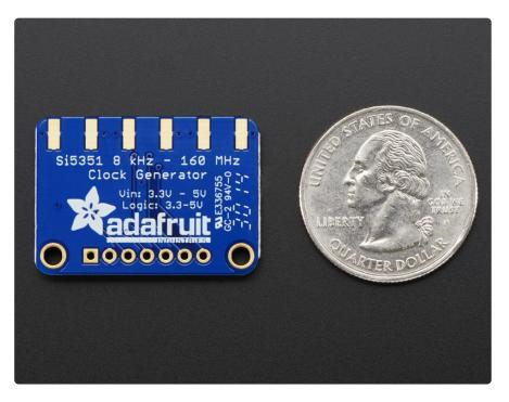
We put this handy little chip onto it's own breakout board PCB, with a 3.3V LDO regulator so it can be powered from 3-5VDC. We also put level shifting circuitry on the I2C lines so you can use this chip safely with 3V or 5V logic.
