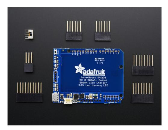
The shield comes as a kit of parts! **Battery is not included, but you can pick one up in the shop**(again, we suggest our 1200mAh battery but you can use any 500mAh+ size you like) There's even an optional switch. If you choose to solder it in, it will let you turn the shield and Arduino power on/off.
