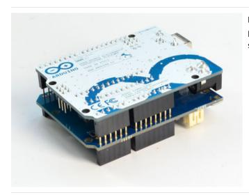
Pull on the shield a bit so that you get a few mm of gold pins showing, then flip it all over and place on a table as shown. It should sit nice and flat
