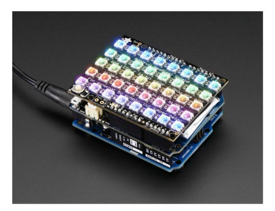
The onboard boost converter can provide at least 500mA current, and can peak at 1A. There's an onboard fuse to protect against higher current draws which could damage the boost converter or battery. The output of the Boost shield is fed directly into the 5V pin on the Arduino, through a protection diode
