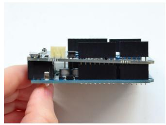
Start by placing the shield on top of an Arduino (any will do) and threading the four long stacking headers through so they plug into the Arduino headers.
