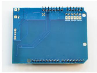
Check your work, especially the power (5V) and GND pads! Make sure there's no bridged solder connections
