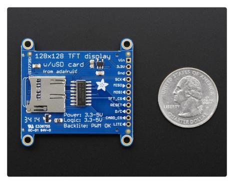
This color display uses SPI to receive image data. That means you need at least 4 pins - clock, data in, tft cs and d/c. If you'd like to have SD card usage too, add another 2 pins - data out and card cs. However, there's a couple other pins you may want to use, lets go thru them all!
