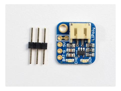
Solder the backpack on with the extra long header so that it can still plug into a breadboard, or clip the long header leads short afterwards for a slim package.
