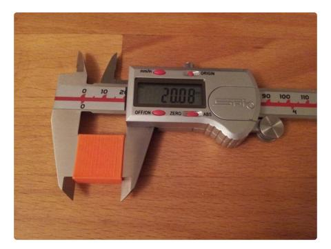
Scale calibration illustrates the process in which you compare the desired dimensions with the actual dimensions your printer produces. The easiest method for accomplishing this is to start by printing a calibration object, like a <u>Calibration Cube</u> (https://adafru.it/cos) or the <u>Calibration Vector</u> (https://adafru.it/cot). Once complete, use a set of calipers to check the dimensions and record your results.
