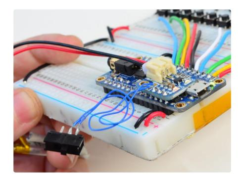
The Lipoly backpack lets you plug in a lipoly battery of any size and recharge it over the MicroUSB connector, so it's basically an all-in-one portable + rechargable system.
