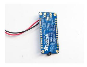
For most battery packs the red wire is the positive wire, connect that to Vin. The black wire is ground, connect that to GND.
