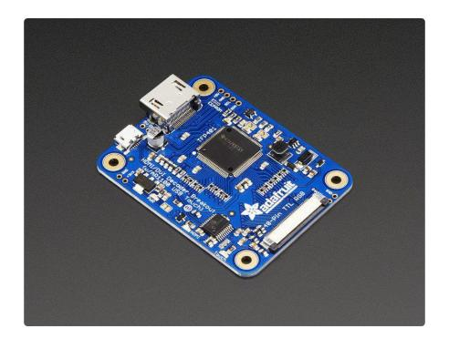
You can even power the display and decoder from a USB port. For example, with a 5" 800x480 display and 50mA backlight current, the current draw is 500mA total. You can reduce that down 370mA by running the backlight at half-brightness (25mA). With the backlight off, the decoder and display itself draws 250mA. If you want more backlight control, there's a PWM input, connect that to your microcontroller or other PWM output and you can continuously dim the backlight as desired
