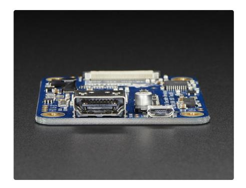
We ship this board with an 800x480 resolution EDID so it will be auto-detected at that resolution. For advanced users, the EDID can be reprogrammed using our example Arduino code. Or, for computers that use linux, you can always just force the resolution to whatever display you have connected.
