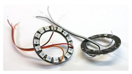
Notice how the wires are inserted from the front, then soldered on the back of the ring. Do it this way if you're new to soldering...it's much easier. It can work the other way too...insert from back, solder on front...but the component tolerances are extrem ely tight and beginners often get a blob of solder in the wrong place and the LEDs don't work.
