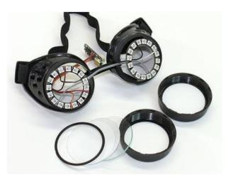
Insert the electronics into the goggles from the front, with the ring-to-ring ribbon cable across the bridge of the nose.
