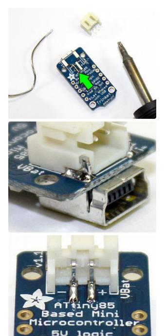
Start by "tinning" one of the JST pads on the back of the Trinket...heat the pad and apply solder so the whole surface is coated.
