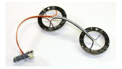
If possible, try to align the rings so they're pointed nearly the same direction (use a landmark like the Adafruit logo for reference). This is not required, but it's a little easier to program animation effects when both rings have the same orientation.
