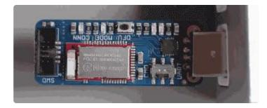
Using your <u>favorite terminal emulator</u> (https://adafru.it/iCU), connect to the BLEFriend at 9600 baud with HW flow control enabled.
