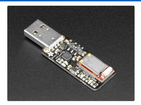
In it's simplest form, it works on the same principle as a common USB/Serial adapter (the FTDI Friend (https://adafru.it/dQa), for example!). Any data that you enter via your favorite terminal emulator on your development machine will be transferred over the air to the connected phone or tablet, and vice versa.
