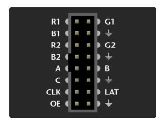
A 32x16 panel uses this pin arrangement. The labels might be slightly different, or the pins might not be labeled at all...but in either case, use this image for reference.
