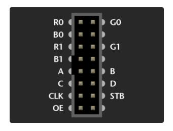
"Variant B" for 32x32 and 64x32 panels. The wiring is identical to Variant A above, only the labels are different.
