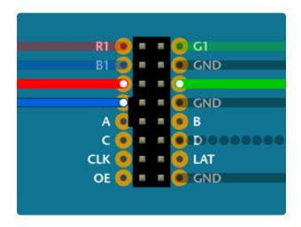
Pins R2, G2 and B2 (labeled R1, G1 and B1 on some matrices) deliver data to the bottom half of the display. These connect to the next three Arduino pins...
