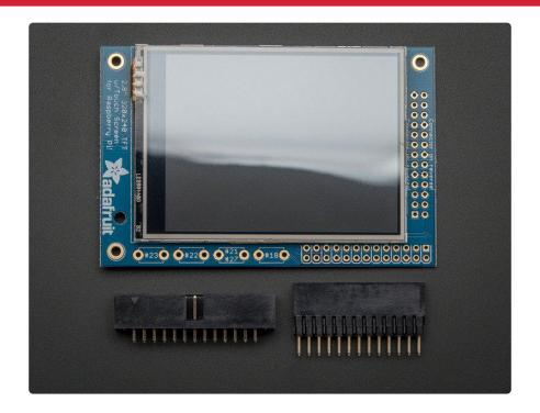
Before you start check that you have the parts you need: an assembled PiTFT plate with the 2.8" screen, extra tall female header and the 2x13 IDC socket. Note that it is normal for the screen to be 'loose' - this is so its easier for you to solder the connector on!
