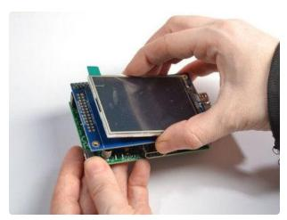
Line up the screen on the white outline, make sure there's some space from the header you just soldered in and the metal sides of the screen. As long as you don't really press down on the screen you can reposition it once or twice.
