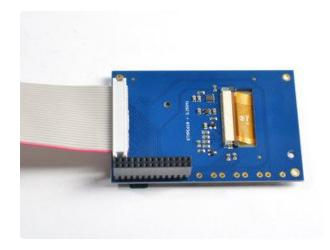
You can attach a 26-pin IDC cable just make sure the pin 1 indicator is on the right as indicated in this photo - there's also a #1 marking on the PCB!
