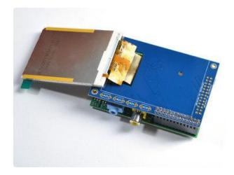
Before attaching the display, check that all the pins are soldered nicely and there's no bridging, cold solder, shorts, or unsoldered pins.
