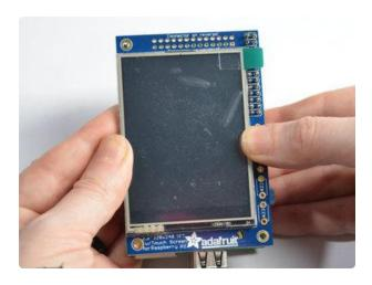
Once you have the screen so it is definitely not touching the header, you can gently press on the sides to secure the tape.
