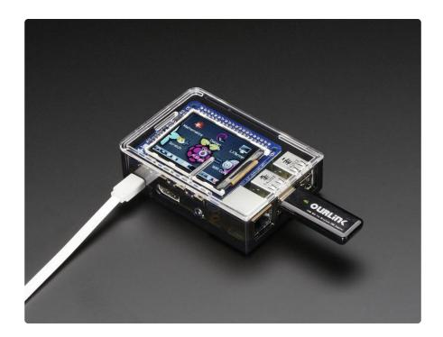
This design uses the hardware SPI pins (SCK, MOSI, MISO, CE0, CE1) as well as GPIO #25. All other GPIO are unused. Since we had a tiny bit of space, there's 4 flat tactile switches wired to four GPIOs, that you can use if you want to make a basic user interface. For example, you can use one as a power on/off button.
