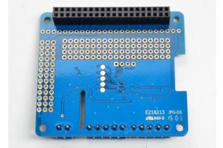
Check over your work so far, make sure each solder point is shiny, and isn't bridged or dull or cracked
