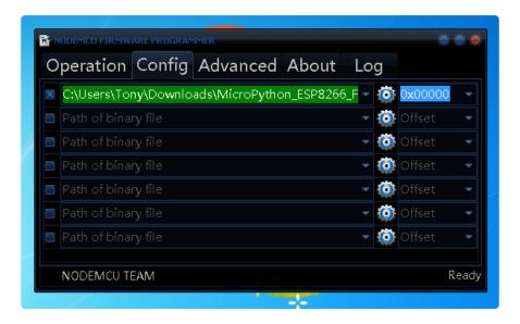
It's very important that your configuration looks like the above with the firmware loaded to offset 0x00000. If you have other firmware files or a different offset then the firmware won't work!
