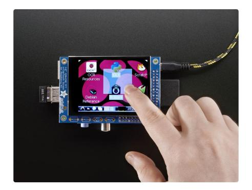
The nifty thing about capacitive touch screens is that they do not require calibration! The calibration is done 'in chip' on the screen itself. However, we still do need to tell the Pi how to read the capacitive chip.
