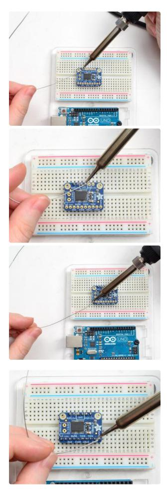
And Solder! Be sure to solder all pins for reliable electrical contact.
