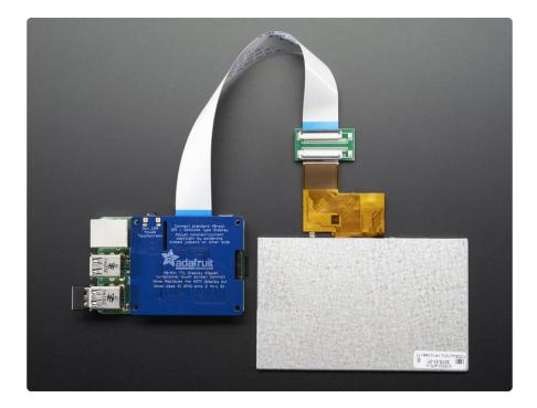
Check the Downloads page for an example datasheet so you can check if your display is compatible. All Adafruit 40-pin TFT TTL displays work, we do not guarantee any other displays work.
