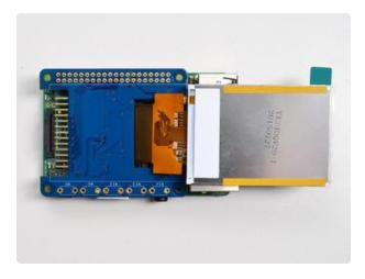
Place the PiTFT HAT on top so all the pins stick through the connector on the side. Gently flip the TFT so its off to the side and wont be in your way while you solder
