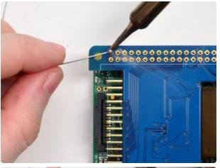
Heat up your soldering iron, and grab some solder. Start by tack-soldering one of the corners. Then you can re-heat that solder point and adjust the circuit board to make it sit flat.
