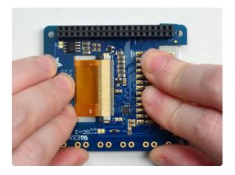
Turn the board over and press gently on the back to get the TFT stuck-on well!
