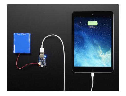
To make this even more useful, we stuck a smart load-sharing Lipoly charger on the other side. The charger circuitry is powered from a microUSB jack, and will recharge any 3.7V/4.2V Lilon or LiPoly battery at 1000mA max rate. There's two LEDs for monitoring the charge rate, a yellow one tells you its working, a green one lights up when its done.
