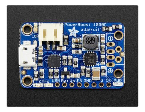
PowerBoost 1000C is the perfect power supply for your portable project! With a built-in load-sharing battery charger circuit, you'll be able to keep your power-hungry project running even while recharging the battery! This little DC/DC boost converter module can be powered by any 3.7V Lilon/LiPoly battery, and convert the battery output to 5.2V DC for running your 5V projects.
