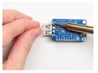
Finally, solder the two mechanical tabs on the side to keep the USB connector solidly in place.
