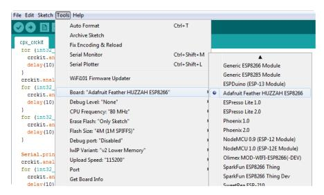
80 MHz as the CPU frequency (you can try 160 MHz overclock later)
