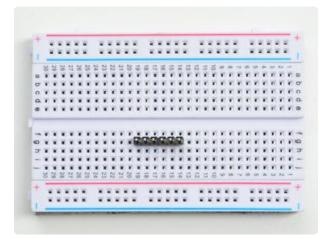
If you're planning on programming with an FTDI or console cable, it's handy to have 6 pins soldered on the end for plugging in.
