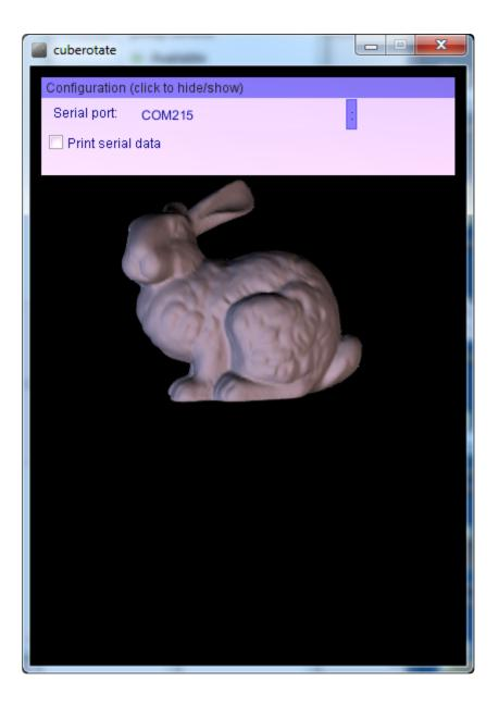
Before the rabbit will rotate you will need to click the : to the right of the serial port name. This will open a list of available serial ports, and you will need to click the appropriate serial port that your Arduino uses (check the Arduino IDE to see the port name if you're unsure). The chosen serial port should be remembered if you later run the sketch again.
