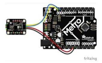
To connect the assembled BNO055 breakout to an Arduino Uno, follow the wiring diagram.
