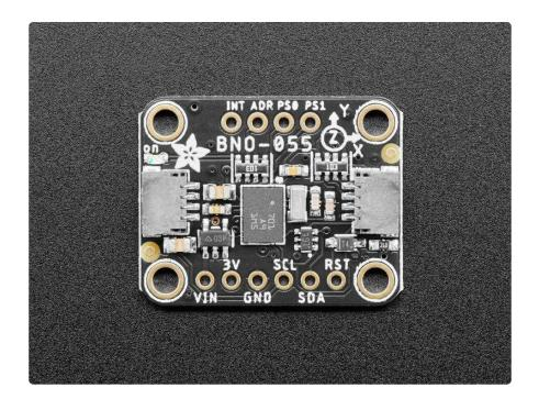
The new version of the board includes <u>SparkFun qwiic</u> (https://adafru.it/Fpw) compati ble <u>STEMMA QT</u> (https://adafru.it/Ft4) connectors for the I2C bus so you don't even need to solder! Use a a plug-and-play STEMMA QT cable to get 9 DoF data ASAP.
