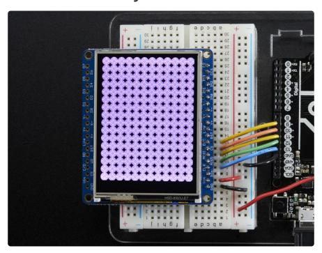
The Adafruit\_GFX library for Arduino provides a common syntax and set of graphics functions for all of our TFT, LCD and OLED displays. This allows Arduino sketches to easily be adapted between display types with minimal fuss...and any new features, performance improvements and bug fixes will immediately apply across our complete offering of color displays.
