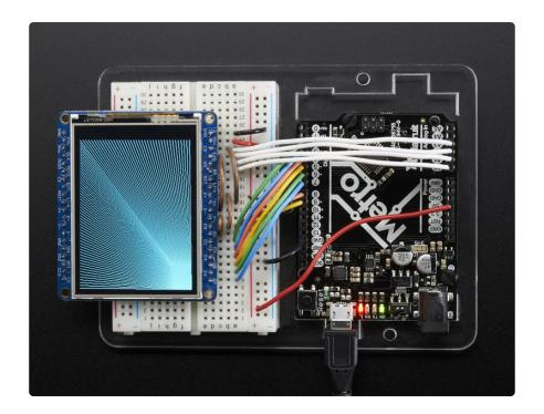
You can connect the seventh pin RST (Reset) to the Arduino Reset line if you'd like. This will reset the panel when the Arduino is Reset. You can also use a digital pin for the LCD reset if you want to manually reset. There's auto-reset circuitry on the board so you probably don't need to use this pin at all and leave it disconnected
