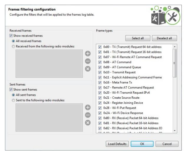
4. Configure the filtering options for one or more of the following: received frames, sent frames, and frame types.
