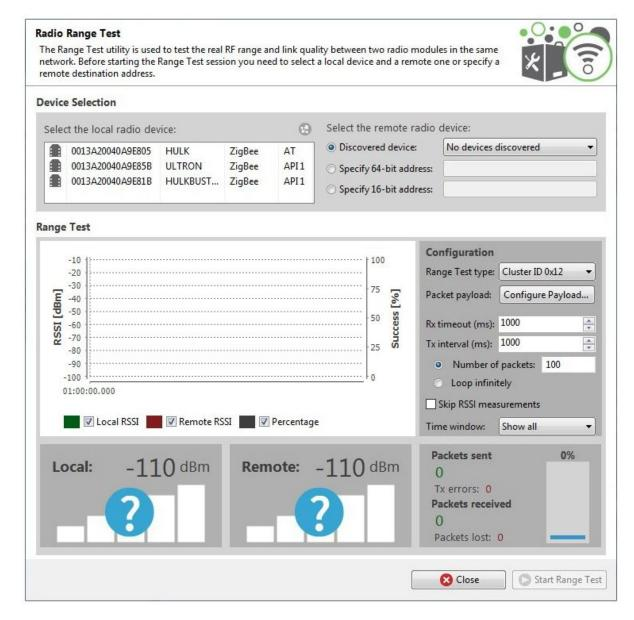
The following sections provide descriptions of the controls and fields in the Radio Range Test dialog.
