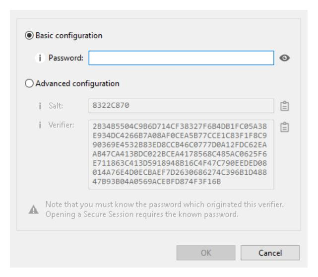
4. In the **Password** field, type the password for the device. As you type, the **Salt** and **Verifier** fields are automatically calculated and populated in the dialog as shown above. This is the password that will be requested when you try to configure the device remotely.
