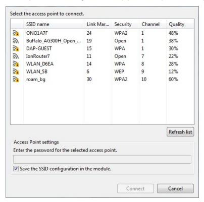
The dialog displays all the nearby access points as well as their security protocols and signal quality. Select the Access Point you want the Wi-Fi module to connect to and, if necessary, configure the password of the Access Point. The Access Point settings also have a check box that allows you to
