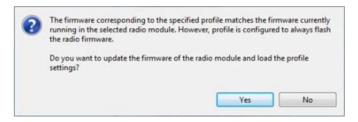
If the firmware of the profile you are loading and the firmware running in the radio module match or the profile is configured to don't flash the radio firmware, XCTU applies the settings saved in the profile to the radio module.
