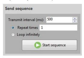
2. Click **Start sequence**. XCTU sends all frames in the **Send frames** list. Sent and received frames appear in the **Frame logs** area.
