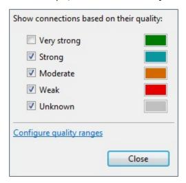
3. Click **Close**. XCTU displays network connections based on the filters you selected. In this example, we can see all of the connections except for those that are very strong.
