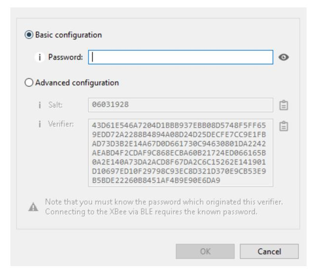
7. In the **Password** field, type the password for the device. As you type, the **Salt** and **Verifier** fields are automatically calculated and populated in the dialog as shown above. This password is used when you connect to this XBee device via BLE using the XBee Configurator app.
