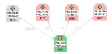
Red radio modules represent devices that were in the network at any time in the past but are unreachable now. When a radio module leaves the network, some devices may still contain information about it. When a new discovery is performed, the module appears to be there but does not answer or is unreachable when XCTU tries to verify the connection.
