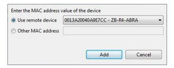
If no remote devices are discovered for the local device, you can enter the MAC address manually:
