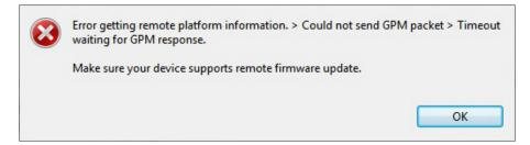
Your remote radio module probably does not support remote firmware update. The following radio modules support the remote firmware update feature:
