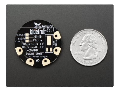
This is the same module and firmware as our BLE UART Friend (http://adafru.it/2479) b ut in a nice rounded shape, so you can switch between the two and have the same working code. This Bluefruit LE does not have the hardware flow control pins so it is best used with a microcontroller with hardware serial support (like, y'know, the Flora!)
