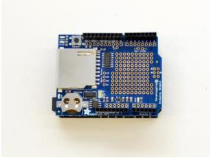
Place the board on the Metro and solder the 2x3 header
