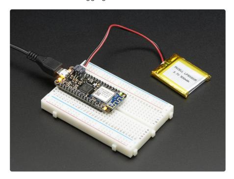
To make it easy to use for portable projects, we added a connector for any of our 3.7V Lithium polymer batteries and built in battery charging. You don't need to use a
