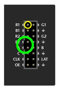
Wires are then soldered from the header to specific Arduino pins on the proto shield. Try to keep wire lengths reasonably short to avoid signal interference.
