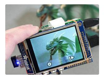
Look at this embarrassing assemblage of rubber bands! There's so much more that could be done here for a proper enclosure...perhaps even laser-cut or 3Dprinted if you have access to such.
