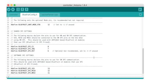
For all the example code, we have at the top of the sketch a few different ways you can communicate with the Bluefruit LE: hardware serial, software serial, hardware SPI and software SPI.
