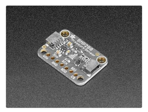
Bosch has stepped up their game with their new BMP280 sensor, an environmental sensor with temperature, barometric pressure that is the next generation upgrade to the BMP085/BMP180/BMP183. This sensor is great for all sorts of weather sensing and can even be used in both I2C and SPI!
