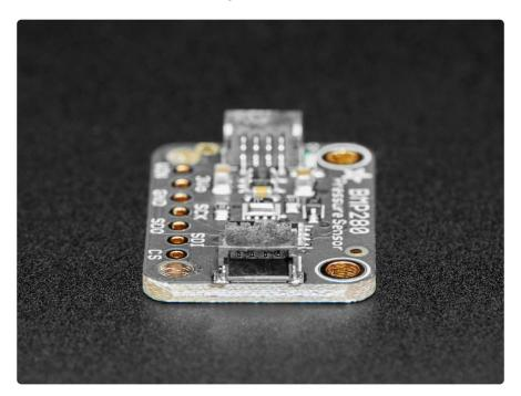
Nice sensor right? So we made it easy for you to get right into your next project. The surface-mount sensor is soldered onto a custom made PCB in the STEMMA QT form factor (https://adafru.it/LBQ), making them easy to interface with. The STEMMA QT connectors (https://adafru.it/JqB) on either side are compatible with the SparkFun Qwiic (https://adafru.it/Fpw) I2C connectors. This allows you to make solderless
