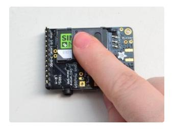
Close the hinge down and slide the cover to lock it in place
