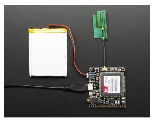
Then press the small **KEY** button next to the battery & cell antenna for 5 seconds. Then the computer will recognize a multi-type USB connection. Install the drivers (https://adafru.it/jFn)
