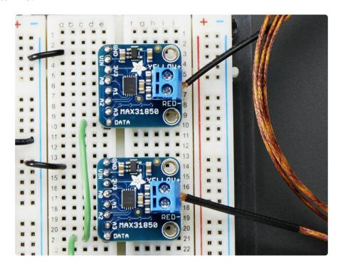
The MAX31850K data format is very similar to that of the well known 1-Wire DS18B20 temp sensor but it is not drop in compatible without code changes to check for the new '1 Wire family' type. We have adapted the classic Arduino <a href="OneWire">OneWire</a> (https://adafru.it/dall) and <a href="DallasTemp">DallasTemp</a> (https://adafru.it/dam) libraries to be MAX31850 compatible, so please click on those links to grab our libraries.
