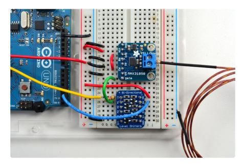
Now if you open up the serial console you should see the OneWire example code print out the data, address and temperature of the sensor. If you mess with the Ax wires you'll see this address value change from 0x00 to 0x0F. This can be a good way to deal with 'hot-swapping' in sensors with unique ROM addresses
