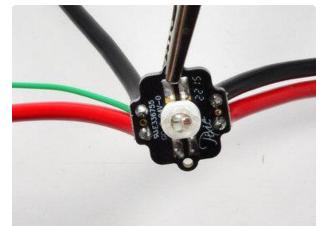
You can use a thinner wire for data, in this case we have a  $^{\sim}22AWG$  data line. It's soldered onto the out pin here
