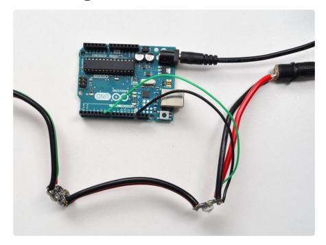
Wiring is easy, you can use any pin with a Serial or Software Serial output pin. We don't use the input of a Serial connection (since the Pixie is 'write only'). Dont forget to power the Pixie with a good 5V supply that can handle the current draw.
