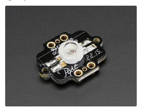
Each Pixie not only contains that aforementioned 3W LED, it also has a Microchip PIC microcontroller. You send it the color you want to appear at standard 115200 baud (1 byte per color). You can send a longer string of pixel data and it will 'forward' along
