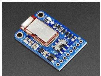
Bluefruit LE UART Friend or Flora BLE If you have a stand-alone UART module you have some flexibility with wiring. However we suggest hardware UART if possible. You will likely need to use the flow control CTS pin if you are not using hardware UART. There's also a MODE pin
