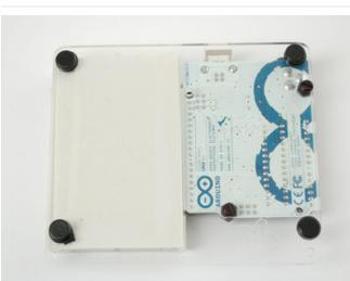
Remove the paper backing from the half size breadboard and stick it on next to the Arduino.
