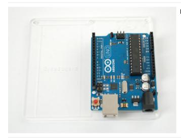
Place the Arduino on top, it should slide onto the bolts
