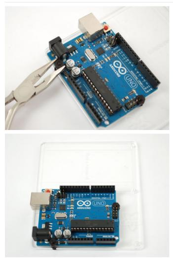
Attach the Arduino securely by screwing on the last two hex nuts
