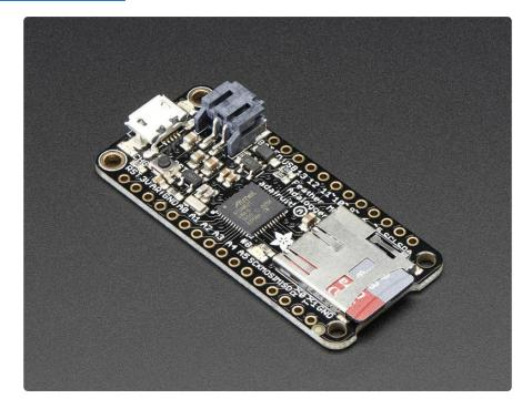
At the Feather M0's heart is an ATSAMD21G18 ARM Cortex M0 processor, clocked at 48 MHz and at 3.3V logic, the same one used in the new <u>Arduino Zero</u> (http:// adafru.it/2843). This chip has a whopping 256K of FLASH (8x more than the Atmega328 or 32u4) and 32K of RAM (16x as much)! This chip comes with built in USB so it has USB-to-Serial program & debug capability built in with no need for an FTDIlike chip.
