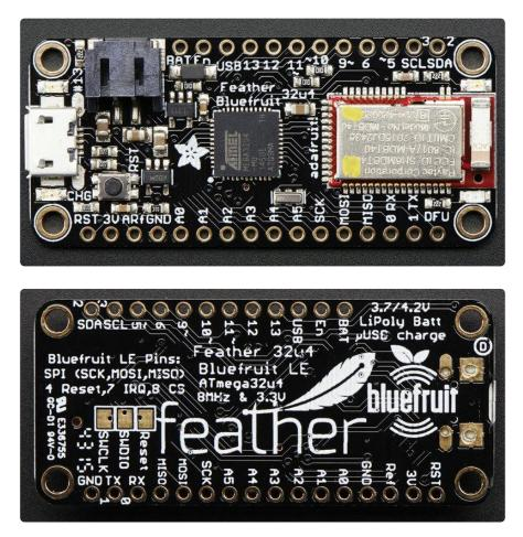
The DFU pin is accidentally labeled GND on the bottom, sorry about that! it should be labeled DFU, dont use it as a GND
