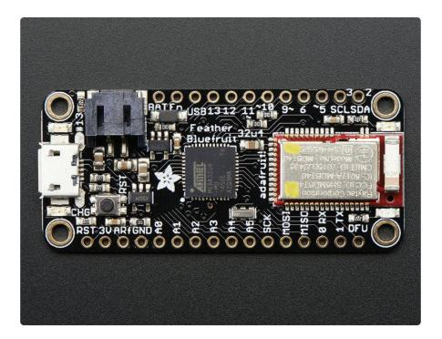
At the Feather 32u4's heart is at ATmega32u4 clocked at 8 MHz and at 3.3V logic, a chip setup we've had tons of experience with as <u>it's the same as the Flora (https://adafru.it/dVI)</u>. This chip has 32K of flash and 2K of RAM, with built in USB so not only does it have a USB-to-Serial program & debug capability built in with no need for an FTDI-like chip, it can also act like a mouse, keyboard, USB MIDI device, etc.
