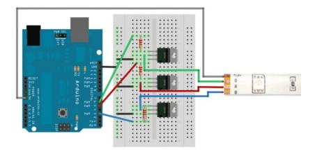
Connect a 9-12V power supply to the Arduino so that **Vin** supplies the high voltage to the LED strip. If you want, you can also just use a separate wire that connects to a power supply that provides about +12V. Make sure to connect the ground of that supply to the ground of the Arduino/MOSFETs!
