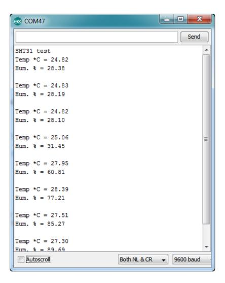
You can try breathing on the sensor to increase the humidity. The sensor reacts very fast!
