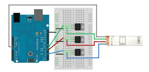
This diagram shows connecting up with power NPN transistors such as TIP120, where Base is pin 1, Collector is pin 2 and Emitter is pin 3. Its very similar except this time we have 100-220 ohm resistors between the PWM output pin and the base.
