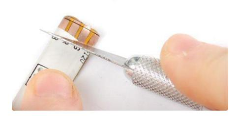
Scrape away the rubber to expose the copper pads.
