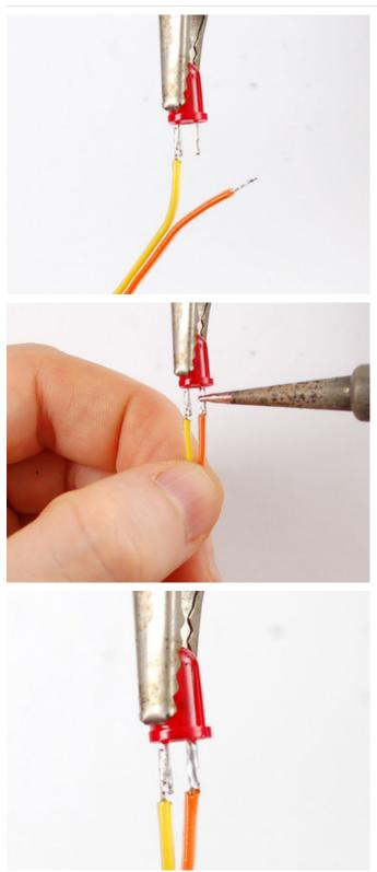
Clip the remaining LED wire and solder the orange wire to it.
