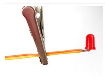
Finally, bend both LEDs (gently and only once) so they are at right angles to the wire. It doesn't matter which way they are bent. The easiest way to do this is to hold the LED in one hand and use a finger to bend the wires.
