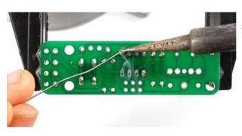
You might want to start by soldering two corner pins. This keeps the socket on straight while you do the rest.
