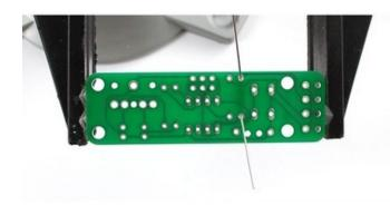
Resistors are **non-polar** which means they don't have a direction: you don't have to worry about putting it in 'backwards' because they work the same either way.
