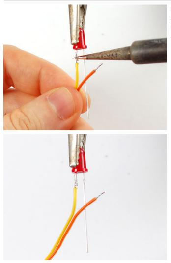
Because there is already solder on the LED and wire, you should be able to hold the yellow wire to the short lead and heat it up with the iron and they'll melt together and hold.
