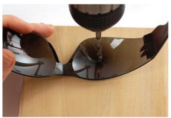
Now we'll drill out the holes for the LEDs to fit in. We used 13/64" drill (0.20 inches / 5.2mm) with great success. You can also try a 3/16" drill bit (5mm) but it may be a little small.
