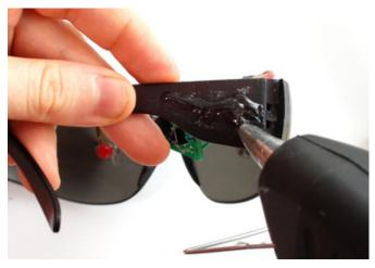
Now we'll attach the PCB. Spread some hotglue, epoxy, silicone adhesive, etc, on to the right arm.
