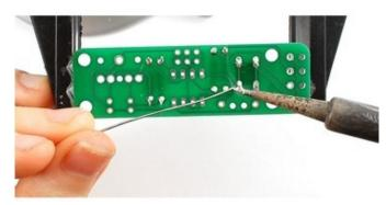
Solder in all four legs of the button. Use plenty of solder because the button needs to be strongly attached to the PCB or it won't work.
