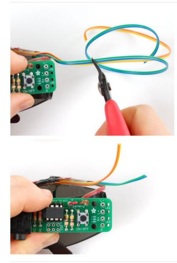
Cut the Orange/Yellow and Green/Blue wires so that there is plenty of slack for them to reach the LED solder holes on the right edge of the PCB. Be sure to have enough wire so that you can fold the arms of the glasses.
