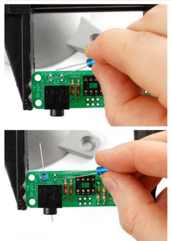
Next are the two electrolytic capacitors **C1** and **C2**. These help smooth the output of the microcontroller audio generation to make it less squeaky.
