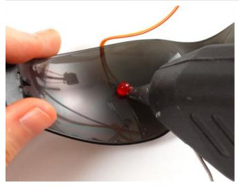
Use hot-glue, white glue, epoxy, silicone adhesive, rubber cement, or your adhesive of choice, to glue the LEDs into place from the inside.
