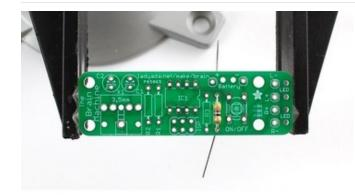
The first part we will place is the resistor **R4** - this is a small oval tan thing with two wires (leads) and color stripes. The stripes are yellow violet black which indicates a 47 ohm resistor. This resistor is used to set the brightness of the lightbulbs (LED) for the right eye. A smaller resistor (less resistance) would make the LED brighter. A larger resistor would make the LED dimmer.
