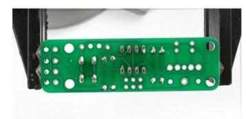
If you mess this up, don't try to desolder the socket, instead just keep going and remember that it is upside down later when it's time to install the chip - the U is just to help you place the chip properly.
