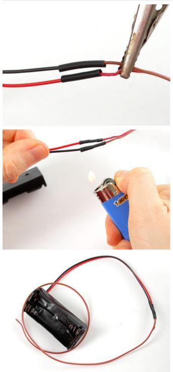
Once the wires are soldered, slip the heatshrink so that it covers the soldered joints.
