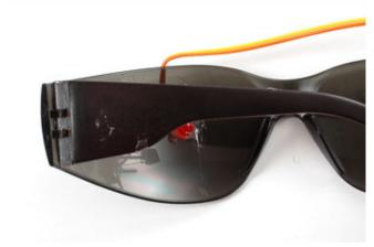
Squeeze a big blob of hot glue on to the left arm of the glasses and stick the battery pack on, making sure that the wires from the battery pack are facing the front of the glasses.
