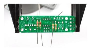
There are another 3 resistors and we'll finish them all up. Place resistor **R3** (another 47 ohm yellow-violet-black) resistor right next to **R4**. This is the resistor that sets the brightness for the other eye's LED.
