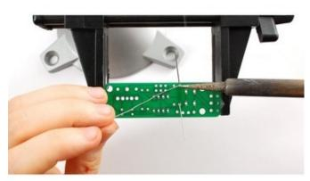
Now you'll solder! Place the flat of the soldering iron tip against the silver ring (pad) and one of the wires of the resistor (lead) at the same time for 2 seconds. This will heat them both up to 600-700 degrees. Then poke the end of the solder so that it flows into the hole and forms a solder joint.
