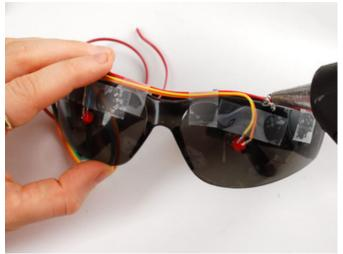
As in the photo, make sure that the arms of the glasses are folded, and use your adhesive of choice to glue the wires to the top of the glasses. The tape will keep the wires in place while the glue hardens.
