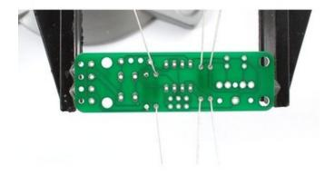
Then place both **R1** and **R2** they are both 2.2K resistors (red-red). These resistors set the loudness of the earphones for either ear. Using a larger resistor (more resistance) would make the volume quieter. Using a smaller resisor would make the volume louder.
