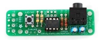
Now we can place the microcontroller chip. This chip holds the brain machine program and is 'burned in' here at the Adafruit factory.
