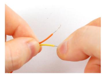
Now we will tin the ends of the wire. Wire needs to be tinned to make good contact. Tinning basically means melting a little solder onto the wires before we attach it to something else. It keeps the strands from flying around and also makes for better solder connection.
