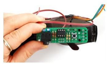
Start with the two power wires (red/brown). Place the PCB on the arm, maybe use tape to hold it in place, and cut the red/brown wire pair so that you have plenty of wire to solder it to the **Battery** terminals (but not so much it's a big mess) -- about 2" extra length is sufficient. (I cut it a little shorter than necessary, give yourself plenty of space!)
