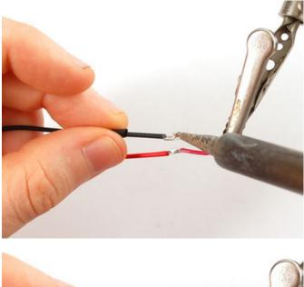
Next solder the black wire to the brown wire. Make sure the heat shrink is on the battery pack wires but out of the way so you don't accidentally heat them up before it's time.
