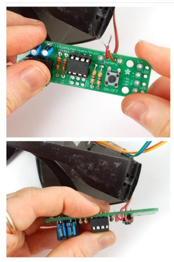
Cut, trim, split, strip and tin the wires. Then slide the **Red** wire through the hole marked + (positive, plus) and the **Brown** wire through the hole marked - (negative, minus).
