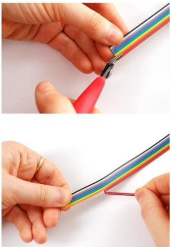
One nice thing about the ribbon cable is that if you clip the wires at the end, you can 'tear' off strips.
