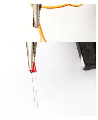
Now we will wire up the LEDs that blink in front of the eyes. LEDs are Light Emitting Diodes - the light emitting part is pretty easy to understand. The Diode part is a little more difficult, but basically a diode is a component that only works 'one way'. Like the capacitors, we have to keep track of which pin is which or the LED won't turn on and light when we want it to.
