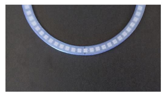
Join the two holder parts together by snapping the tabs on the ends together. Carefully insert the 60 NeoPixel ring into the assembled holder. Thread the wires through the hole of the neoring-60-bottom.stl and out the hinge connector.
