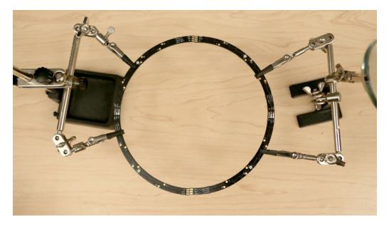
With two halves soldered together, you can orient the ring and the third-helping hands to a comfortable position. Align them up as best as you can and solder these together.
