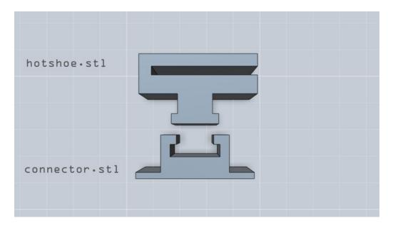
Firmly slide the **hotshoe.stl** part through the **connector.stl** part were the two sides interlock. The small "T" shape on the side of the **hotshoe.stl** part meets with the "C" shape of the **connector.stl** part.
