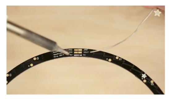
Start by soldering just two pieces together. Once you've aligned them up, apply a line of solder from one connection to there other. Make two sets of halves and solder those together.
