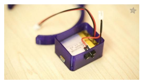
Plug the battery into the JST extender and insert the slide switch through the top opening by pressing it through the top hole of the enclosure.
