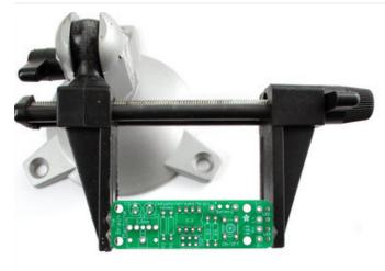
Place the PCB in a vise (if you have one), and turn on the soldering iron. Make sure you have all the tools you'll need to assemble the kit. (https://adafru.it/c1y)
