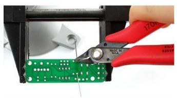
Now we will get rid of all that excess wire. Use your diagonal nippers to clip the wire just above the end of the solder joint. there should be almost no 'wire' sticking out.
