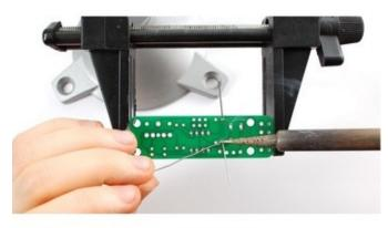
Once you are happy with the first solder joint, solder the other resistor wire.
