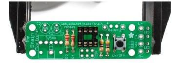
Now we will place the chip socket. A socket is a protector. In case you want to replace the chip or it gets damaged, or something, it's important to have it in a socket. That way you don't have to permanently solder in the chip.
