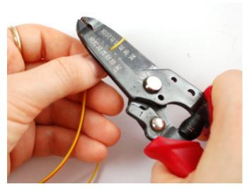
Strip the wires about 1/2" (1cm) away from the end, using any kind of wire strippers. If you mess up and cut the middle wires, just cut the wires short, tear them apart and try again. You have a lot of wire so there's plenty to practice with.
