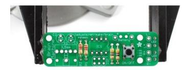
Next is the tactile button that is used to tell the microchip in the kit to turn on and off. The button is also nonpolar (it's just a mechanical switch) so you cant put it in 'backwards' It should snap into place right next to the **ON/OFF** silkscreen label on the PCB.
