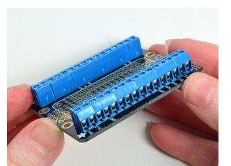
Place the two strips on either side of the breakout PCB with the terminal block holes facing out
