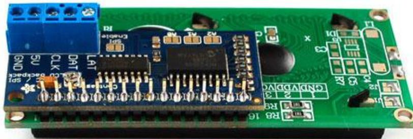
Make sure that as you solder the first pin, the backpack PCB isn't leaning against the LCD, where the terminal blocks could short against some components. You can put some electrical tape or foam tape behind to avoid this if you think it could be an issue.
