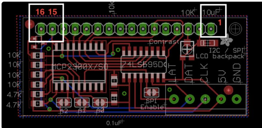
If your LCD has 18 pins, you won't be able to use the extra backlight pins, just connect 1-16 and leave 17 and 18 disconnected
