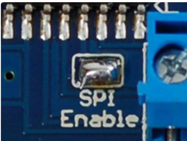
Don't forget to solder closed the SPI jumper on the board if using the SPI wiring!
