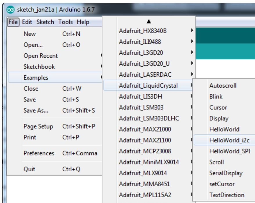
Upload the sketch. You should see the backlight turn on when the Arduino resets. If you don't see any characters, adjust the Contrast trim potentiometer with a mini-screwdriver until you see the text clearly
