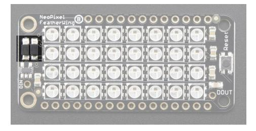
That means, if USB is plugged in, you'll get ~5V USB power. If the feather is running off of battery power, say a LiPoly battery, you'll get 3.7-4.2V power. While this is a little lower than spec, NeoPixels are only a little dimmer.
