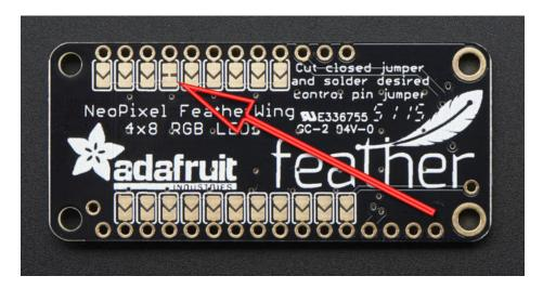
This pin is #6 for Feather 32u4, 328p, M4, nRF52840 and M0s, and is #16 on ESP8266 Feather.
