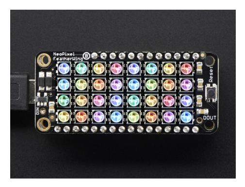
Put on your sunglasses before staring into these 32 configurable eye-blistering RGB LEDs. Arranged in a 4x8 matrix, each pixel is individually addressable. Only one pin is required to control all the LEDs. On the bottom we have jumpers for the DIN line to any of the I/O pins on a Feather. You can cut the default jumper trace and use any pin you like. (In particular, the default pin for Feather Huzzah ESP8266 must be moved, try pin #15!)
