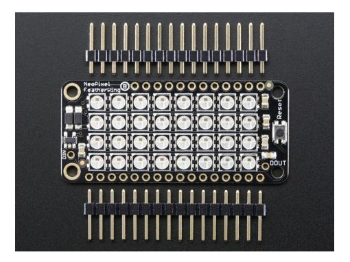
A level-up shifter converts the 3.3V logic of the Feather to the power line voltage. If, say, you need MORE blinky, you can chain these together. For the second Wing, connect the DIN connection to the first Wing's DOUT. Also connect a ground pin together and power with an independent 5V supply to keep from loading the power supply too much.
