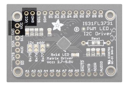
You can power the IS31 from 2.7-5.5VDC, but note that the same voltage is used for both power and logic.
