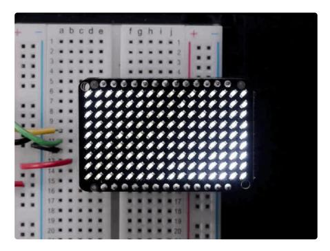
This chip is great for making small LED displays, and we even designed the breakout to match up with our ready-to-go LED grids in red, yellow, green, blue and white. Sandwich the driver and matrix breakout, solder together for a compact setup. Or you can DIY your own setup, just follow the LED grid schematic in the IS31FL3731 datasheet.
