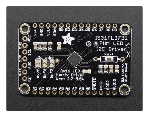
The IS31FL3731 has a lot of pins, and we wanted to make it easy to use with a breadboard while sandwiched with an LED matrix. The easiest way we could figure out to do this is make the board as large as our 0603-LED 16x9 matrix grids and have a control header on one edge. That way you can solder the two long headers directly to the matrix and still have access to pins for power and data.
