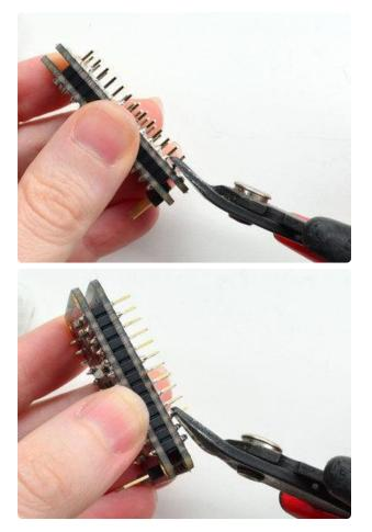
Now you can trim the long header with diagonal cutters. Cut one or two pins at a time
