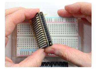
The LEDs face out and connect to the two side header strips.
