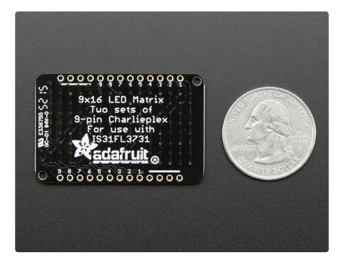
Pick up a driver board and your favorite color LEDs to match. You'll need to do some basic soldering to attach the driver backpack and matrix together, and run wires to your microcontroller, but its not too hard. Then install our Arduino code to get some LEDs blinking immediately. Our library is Adafruit\_GFX compatible so you can draw lines, circles, text, and small bitmaps if you want more graphics control
