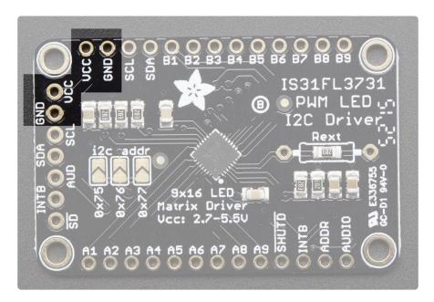
You can power the IS31 from 2.7-5.5VDC, but note that the same voltage is used for both power and logic.
