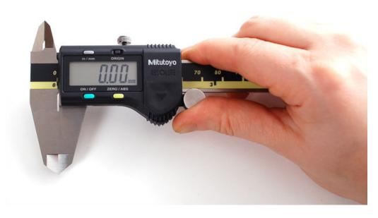
Before using your calipers, check that the origin is correct, clean the blades with a cloth to make sure there's no dust or dirt that would give the wrong measurement and close the jaws. You should read 0.0mm, if not, check that they're clean and if so, press the **origin** button. We've never had to do this since they are pre-origin'd at the factory but hey, you never know.
