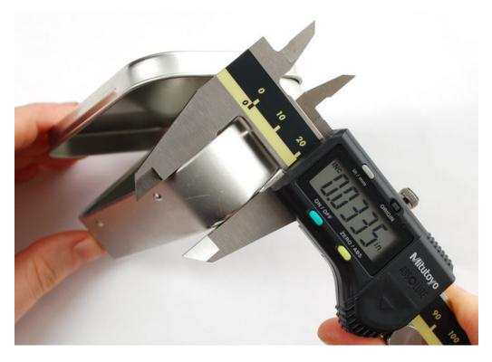
This measurement came out to 33.5 mils. The closest standard sheet gauge (https://adafru.it/aJ8) to 0.0335 is 20 gauge. Variations in the metal thickness may be due to additional thickness from the plating process or the rounded edges interfering with the depth measurement. Taking multiple measurements is always a good idea!
