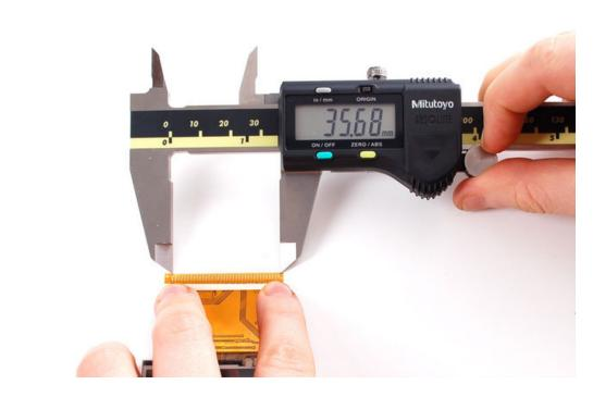
Remember that for a N pin connector, there are N-1 'gaps' (a common-enough confusion that it has its own name, the fencepost-error (https://adafru.it/aJ9) ) so divide 35.68mm by 36 = 0.99mm. Since we're eyeballing the center points of the connector, this should be rounded up to a 1mm pitch. Sometimes the number should be rounded up/down in imperial so if it seems off, check other units.
