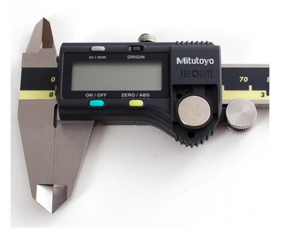
Digital calipers do require a battery (there are solar ones as well, with an internal backup battery) but good calipers rarely need to have the battery replaced. The pair we have is used many times a day and often isn't even turned off for a few days but has been running without issue for over 5 years. We do suggest turning them off when not in use but many people don't even bother since the battery drain is so low.
